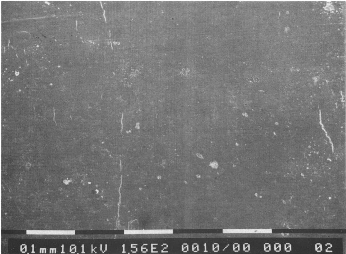
Fig. 8. Surface of poly(L-lactic acid)-gentamicin sulfate (33% w/w) implants before dissolution, magnification 156 ×.
